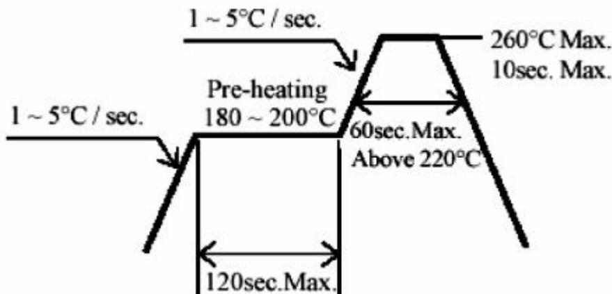
3.2 When soldering, do not put stress on the LEDs during heating. 焊接时, 加热期间不要对按压 LED.
